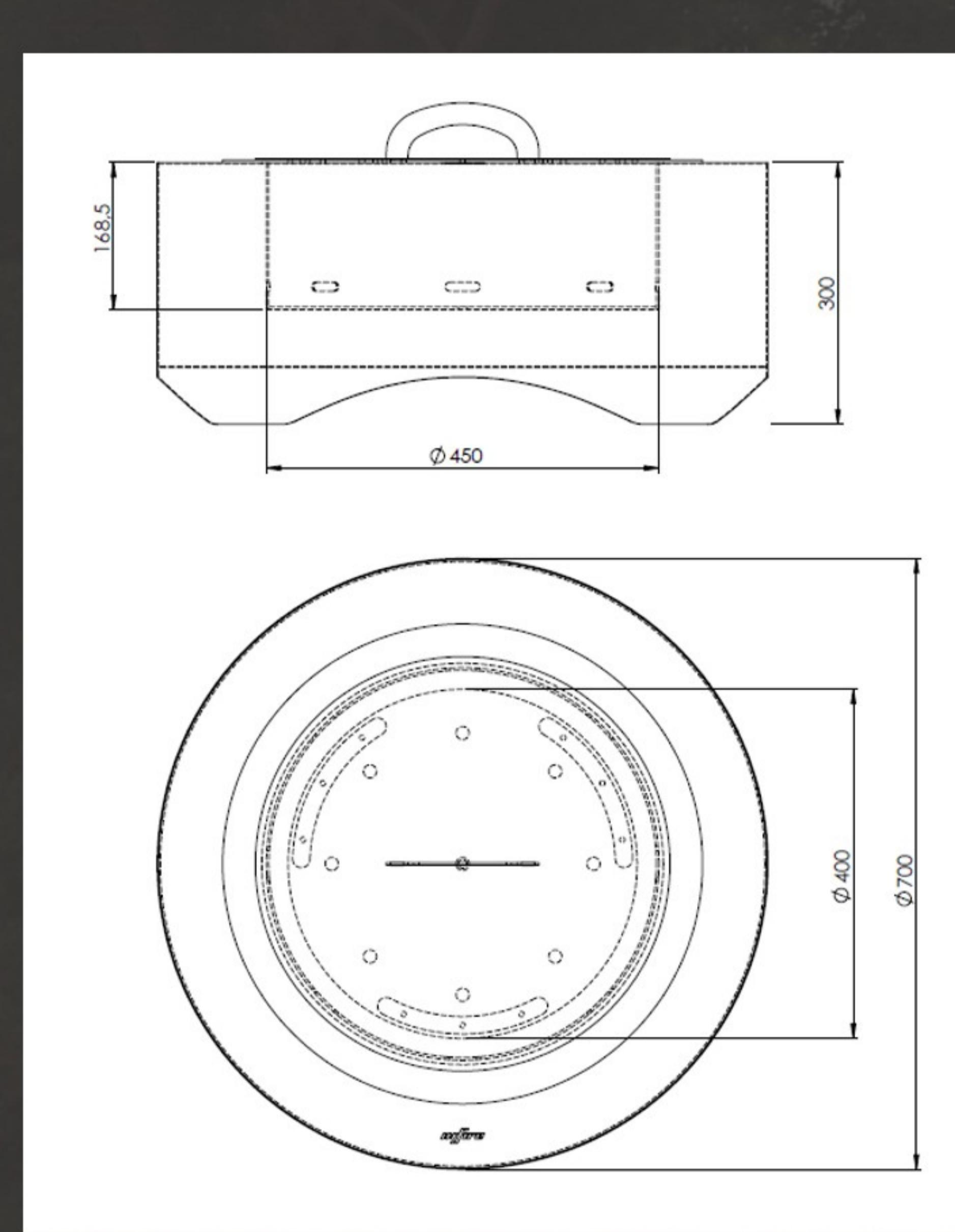
A round fireplace with a housing, insert and cover. Housing made of 1.5 mm thick steel. The insert is 3 mm thick and covered with a special paint resistant to very high temperatures. The set also includes a cover with a handle with a steel thickness of 1.5 mm, enabling safe storage of the fireplace and protecting against the spread of embers or ash./
